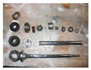
Once the nut is removed the rest of the piston assembly can be dismantled.
