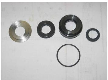
The original seal and top washer are discarded and replaced by a new seal head and lower washer. The seal head accepts a new seal and a wiper. An O ring is used to seal the OD of the seal head.
