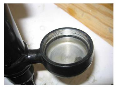
Install a new O ring (cross section 2.0mm Inside diameter 43.5mm, standard size S44) into the lower bladder housing. Lube O ring with SAE 5 shock oil.
