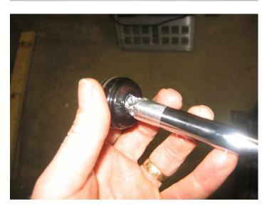
Wrap the end of the chrome tube in a single layer of aluminum tape to protect the seal from the sharp edges. Dip the wrapped end in shock oil to fully wet it then carefully work it through the new seal assembly. Remove the aluminum tape once the seal is on the shaft.
