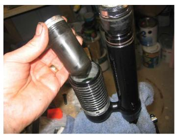
Insert cleaned bladder into bladder housing. Oil should overflow around bladder before it is fully inserted to ensure no air is entrapped. Add more oil to housing if necessary.
