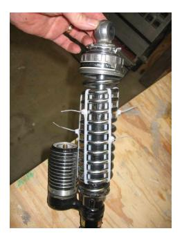
Then back off the spring adjuster to fully unload the spring and remove the cap etc.
