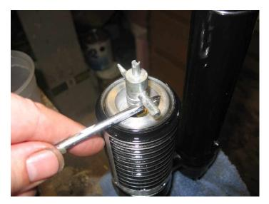
Pull bladder back up using valve tool or remove Schrader valve and screw a bolt into threads to pull with.
