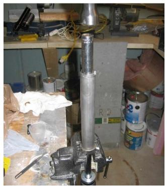
Tap the assembly fully together by standing it up in open vice jaws and using a socket to apply the hammer force to the end of the tube assy.
