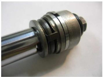
View of piston end. Note the parts are pretty much Poke Yoke and only assemble one way.
