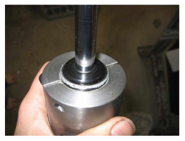
Edge fully crimped over. Need to fix the paint now.
