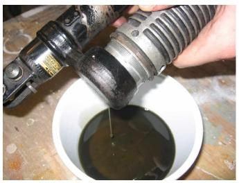
Oil will come out. I collected two shocks worth of oil and tested it by recording the time for a measured amount to flow through a fixed orifice. It came out as very slightly lighter weight than SAE 5 fork oil. I am guessing the viscosity drops a fraction with use and age so I use SAE 5 oil to refill units.
