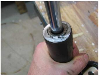
You need to grind away enough until you see the witness mark of the tube ID. The tube wall thickness is 1.5mm. This requires grinding a little below the top surface of the washer. In this picture I did not go quite far enough.
