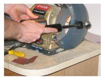
Take body of shock to bench grinder or belt sander and grind away rolled over crimp on top surface. BE VERY CAREFUL not to touch piston rod as any damage to this will make it useless.
