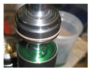
Finish with the cylinder full to overflowing with no more air bubbles coming up. Remove the Schrader valve core and lower the seal head into the end of the tube. The reason to take out the valve core is to deplete any internal pressure as the cap goes in. if you don't do this it can ride back up again.
