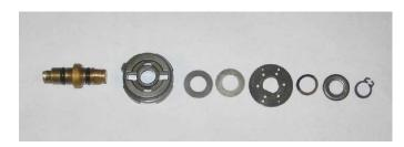
The valve assembly is held together with a snap ring. Once this is removed it can be dismantled cleaned and reassembled. The O rings are Metric size: section 1.5mm Inside diameter 5.5mm
