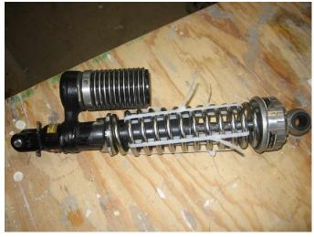
To remove the coil spring I use zip ties as spring compressors. Start with the spring adjuster set to its highest setting then compress the coils with 5 or 6 zip ties. After they are all in place you can work round and round pulling each one a bit tighter.
