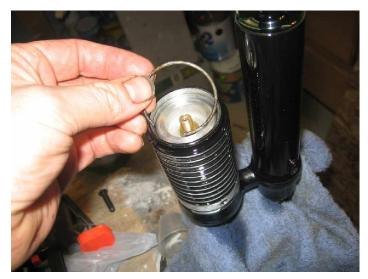
Press bladder assy down far enough to uncover snap ring groove. Install snap ring.
