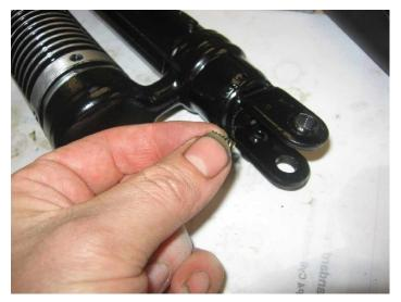
Install spring into bottom of housing and stand housing vertically in a vice.
