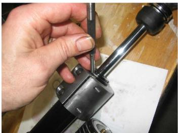
I made up a clamp block to support the tube wall while staking over the edge of the tube using a hammer and punch. I found the best method was to have a helper hold the shock body horizontally and slowly roll it along while I did the tapping.
