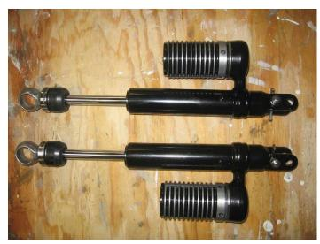
Reinstall Schrader valve core and inflate bladder to 28psi. Work shock back and forth by hand checking function of adjusters and for any oil leaks. Let sit for 24 hours and recheck air pressure. It should not leak down.
