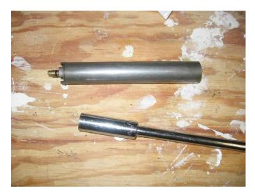
Now use a 14mm socket with an extension attached or similar piece of tube to reach down inside the piston tube. Make sure socket or tube has a smooth flat end with no lumps or burrs on it.
