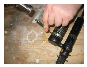
Use a suitable wrench (or punch and hammer) to loosen the lock nut that secures the nitrogen bladder housing.
