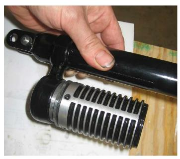
Wipe end of bladder housing that engages with O ring with SAE 5 shock oil. Then ensuring lock nut is in place screw bladder housing into shock body. Screw fully in then back out to align vertical ribs on housing to face fore and aft. Tighten lock nut.
