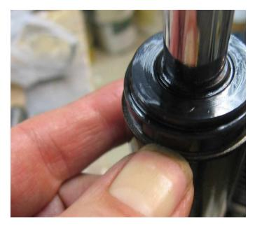
Carefully work around the seal with a thumb nail or similar to ease the seal down over the edge of the tube. (This is where the seal will get cut if you did not previously smooth of the sharp edge and remove any burrs). Press the seal cap down gently while working the O ring into place. Once O ring is below the edge of the tube press the seal head fully down into place.
