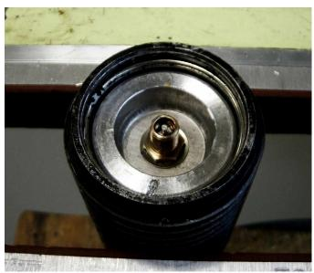
Once it is pressed in far enough, hook out the snap ring. Then either screw a valve tool onto the Schrader valve to pull with or unscrew and remove the Schrader valve, then screw a bolt into the threads. Pull bladder assembly out.
