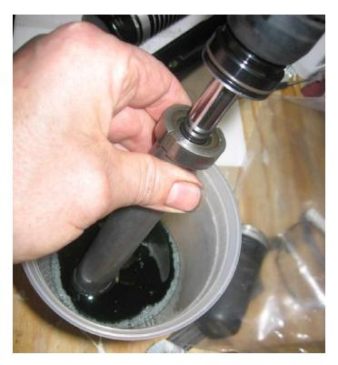
Immerse end of shock assembly in SAE 5 shock oil and pump unit up and down until oil is pumped out around bearing. Keep pumping until the oil coming out is free of air bubbles.
