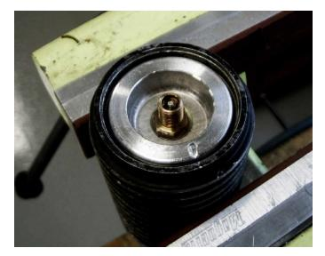
Hold the canister in a soft vice and press the aluminum center down to expose the snap ring retaining it. Use a socket of suitable diameter and C clamp to do the pressing.
