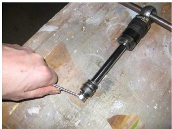
To disassemble the shock rod, hold the top eye with a bar and use a 10mm wrench to undo the bottom nut. This nit was staked in place so a tread or two will be broken off as the nut comes undone. Note the retract buffer is missing from this picture as it got trashed during a disassembly learning process.
