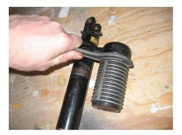
Use a pin wrench (or hammer and punch) to loosen the bladder housing then fully unscrew and remove the housing.
