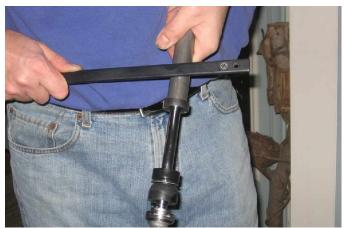
Separate the damper assembly by tapping the upper bearing cap off the end off the damper tube. A flat steel bar or similar type device is best suited for this. Tap one side then the other to pull it off squarely.
