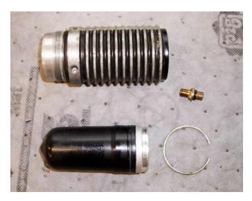
Thus. Now is a good time to clean and paint the aluminum housing. Screw the Schrader valve back into the bladder to keep crud out.
