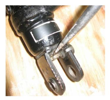
Use a flat screw driver as a pry bar to lever off the damper adjustment. Note as this comes off a ball bearing will fall out. You will see a spring in the recess behind where the ball was but this can't come out until the shock is pulled apart.
