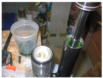
Top off the oil in the main cylinder and then carefully work the piston up and down about ½" at the top of its stroke while topping up the oil. This is to work the last of the air out. Lower the seal washer down over the bearing housing.
