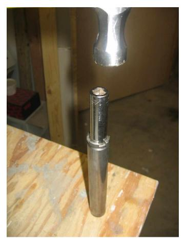
Once the valve has been cleaned and rebuilt it can be tapped back into the end of the cleaned tube. I used a ½" socket here.
