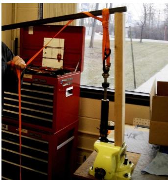
Use some kind of lever device to pull the shock apart. If you did not grind off enough in the previous step the shock wont pull out but the force you apply trying will trash the 'up stop' buffer inside the shock. It does take some effort to pull the shock apart but you should see the witness on the ground face showing almost immediately. Watch out for oil to come out the bottom as the shock pulls apart.
