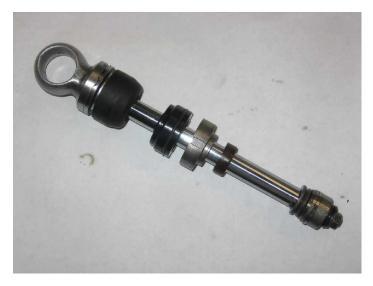
Reassemble piston rod assembly with new seal and bearing. Note this pic shows an earlier seal option and the washer that is located between the seal and end cap is missing.
