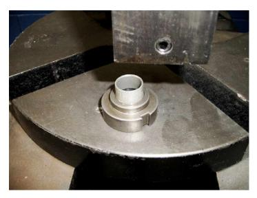
Press in a new bearing. Oil the OD of the bearing and the bore prior to pressing it in.
