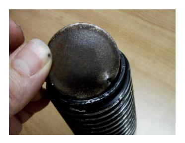
First job is to remove the thin metal cap from housing gas canister housing by prying out. I have not found a good way to get it out without damaging it yet. Depress the Schrader valve underneath to dump any air pressure.
