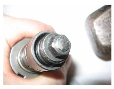
Check for free movement of the compression adjuster and if OK, beat the end of the rod over with a hammer to fully secure the nut. Wipe off any excess loctite.
