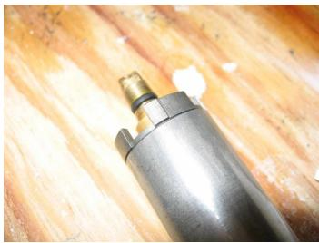
Note the small lug on the side of the valve body. Look down inside the main shock body and you will see a recess at the bottom that this needs to engage into. Slide the tube assembly into the shock body. (The O ring should be nicely lubed from the previous operation).
