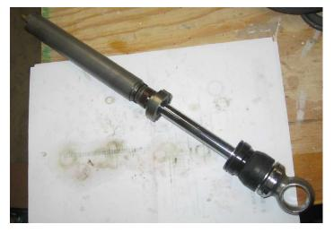
Lube the ID of the tube and piston rod end with SAE 5 shock oil. Insert rod assembly into tube compressing the piston ring to get it started.
