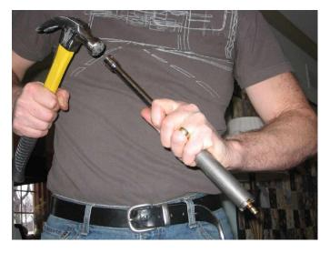
Hold the shock tube in one hand and use the socket to drift the valve assembly out of the end of the tube. The impact is applied to the face of a valve washer that must be flat to work properly. I trashed my first one using a pin drift which put a dent in the washer.
