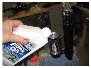
Once piston assembly is fully pressed down, Check that the little spring is still in the housing at the bottom. (If not you will have to pull the assembly back up a bit to reinstall the spring). Now half fill bladder housing with SAE 5 shock oil and gently work piston up and down a few times while holding top bearing down with a screw driver tip or similar.
