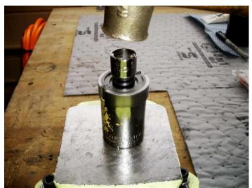
The DU bushing can be removed from the upper bearing cap by tapping it out with a 15mm OD socket or similar rod or tube.
