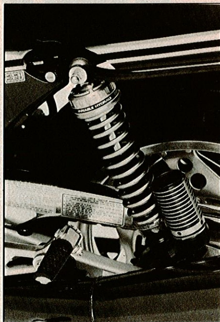
Both compression and rebound damping are adjustable by hand; springing is firm.
