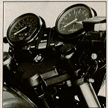
Damping adjusters sit on top of fork legs; air valve on right leg links both legs.
