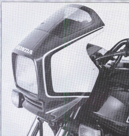
The miniature fairing doesn't provide much wind protection, but it does smooth airflow.
